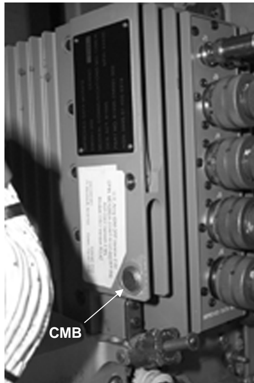
Figure 117. Improved Data Modem (AH-64A/D) with CMB Installed
