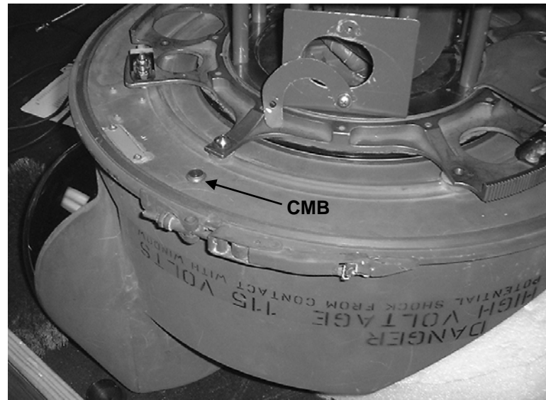
Figure 181. PNVIS Turret (AH-64A/D) with CMB Installed
