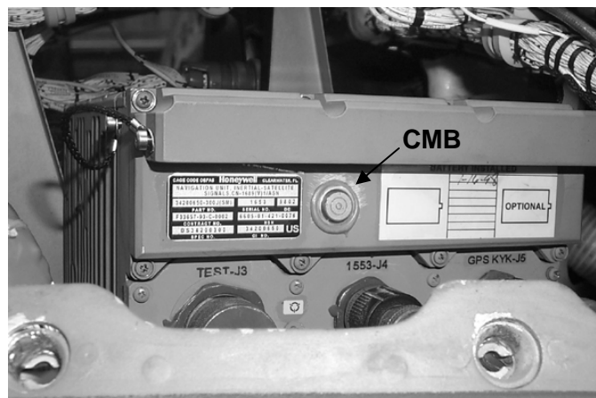
Figure 115. Inertial Navigation System (AH-64D) with CMB Installed
