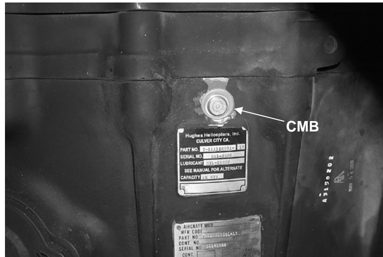
Figure 51. Main Transmission Assembly (AH-64A/D) with CMB Installed
