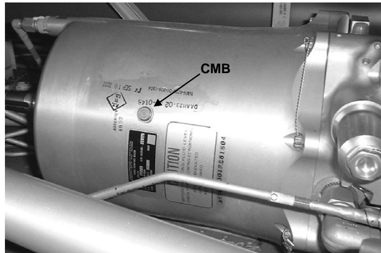
Figure 68. Hydraulic Manifold, Utility (AH-64A/D) with CMB Installed
