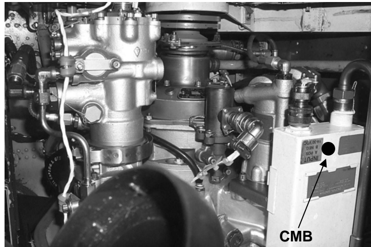
Figure 104. Auxiliary Power Unit (AH-64A) CMB Location
