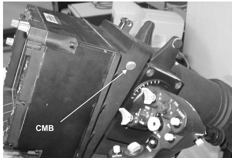
Figure 173. TEDAC Sub-Assembly (AH-64A/D) with CMB Installed
