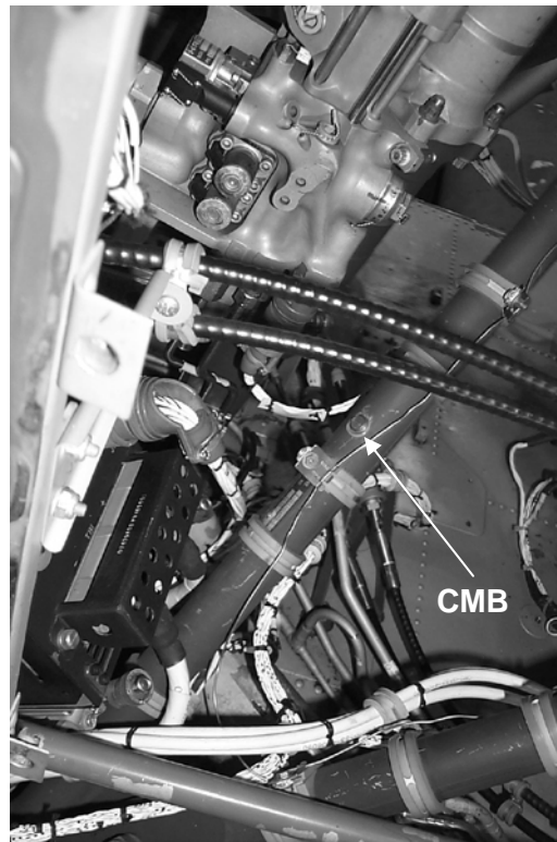
Figure 11. Center Strut (AH-64A/D) with CMB Installed
