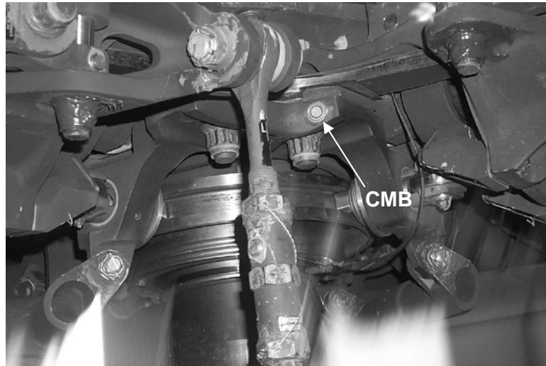
Figure 29. Lower Shoe Assembly (AH-64A/D) with CMB Installed
