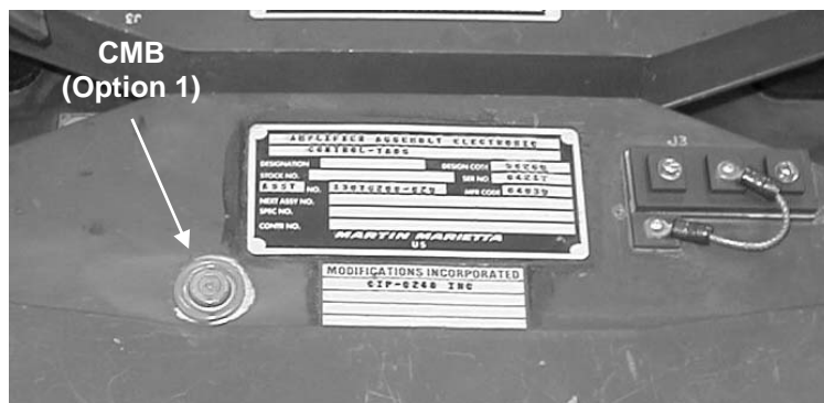
Figure 141. TADS Servo Electronic Torque Amplifier (AH-64A/D) with CMB Installed
