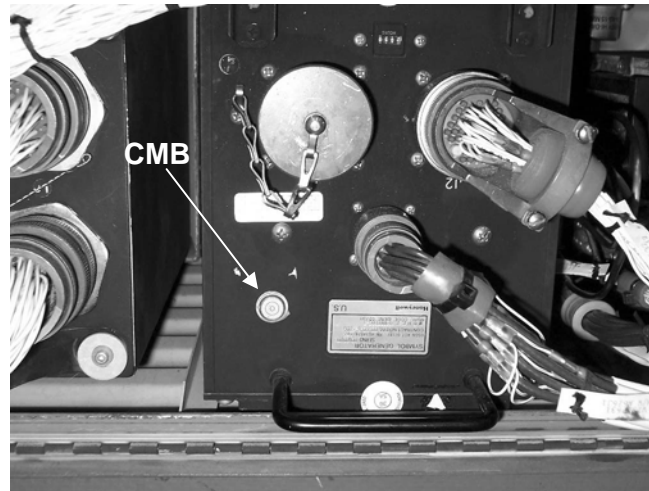
Figure 195. Symbol Generator (AH-64A) with CMB Installed
