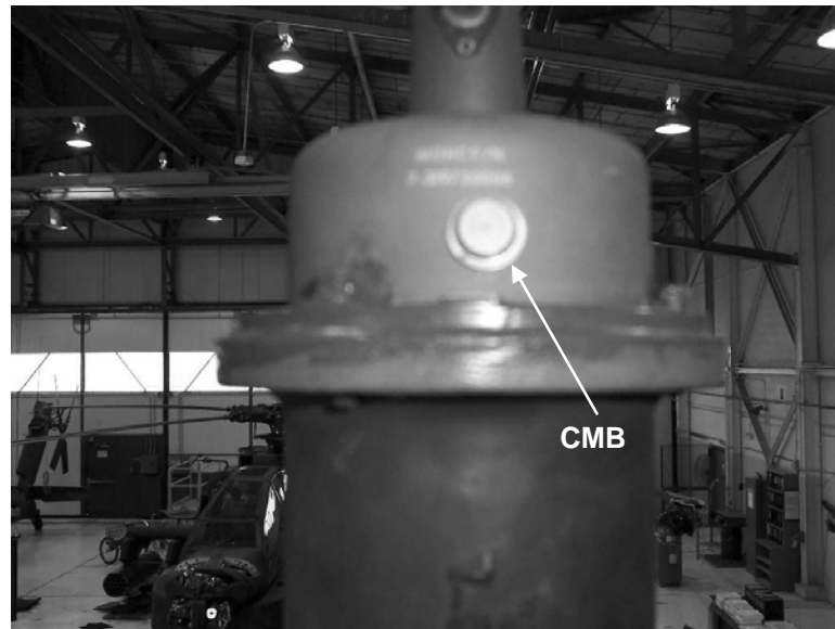
Figure 123. Omnidirectional Airspeed Sensor (AH-64A) with CMB Installed
