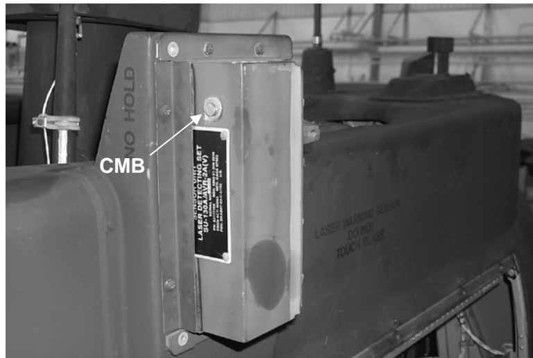
Figure 206. Laser Sensor Unit (AH-64A/D) with CMB Installed
