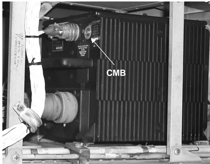
Figure 112. Signal Data Converter (AH-64A/D) with CMB Installed
