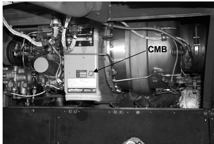
Figure 106. Auxiliary Power Unit (AH-64D) with CMB Installed
