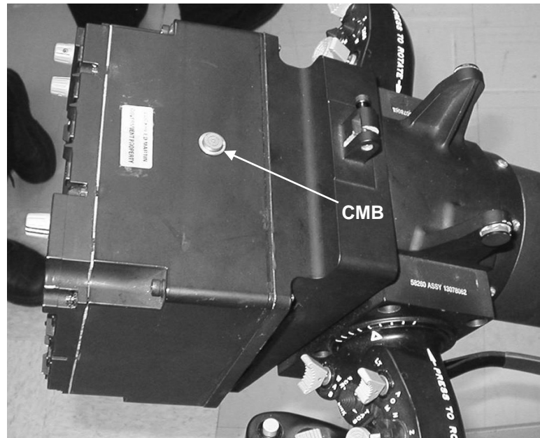
Figure 179. TEDAC Display Unit (AH-64A/D) with CMB Installed
