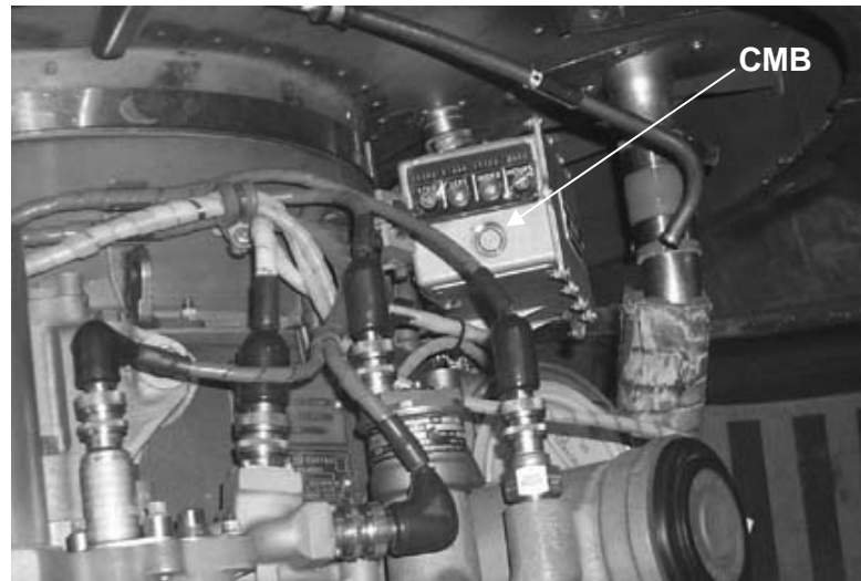
Figure 19. Engine History Recorder (AH-64A/D) with CMB Installed
