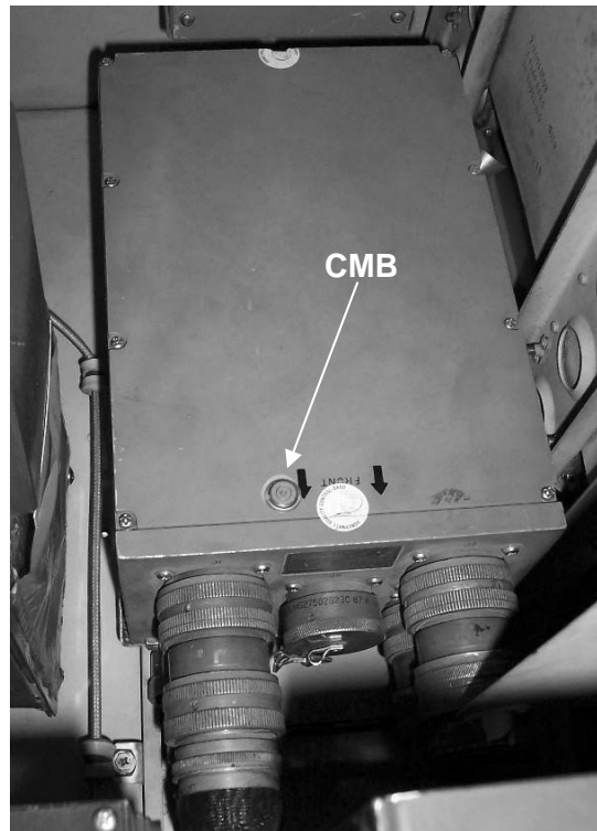
Figure 100. DASE Computer (AH-64A) with CMB Installed
