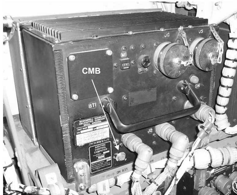
Figure 121. Fire Control Computer (AH-64A) with CMB Installed
