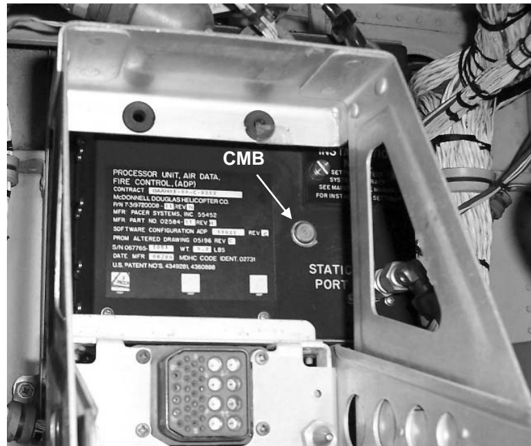
Figure 125. Air Data Processor (AH-64A) with CMB Installed
