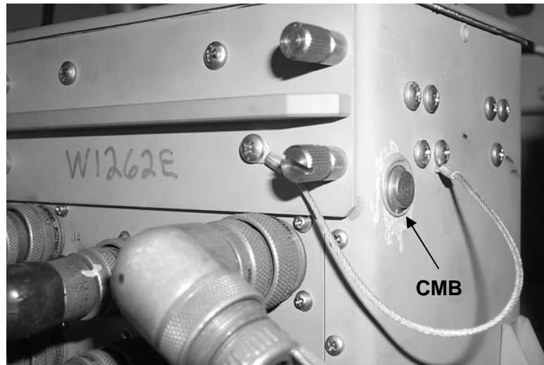
Figure 208. Comparator (AH-64A/D) with CMB Installed
