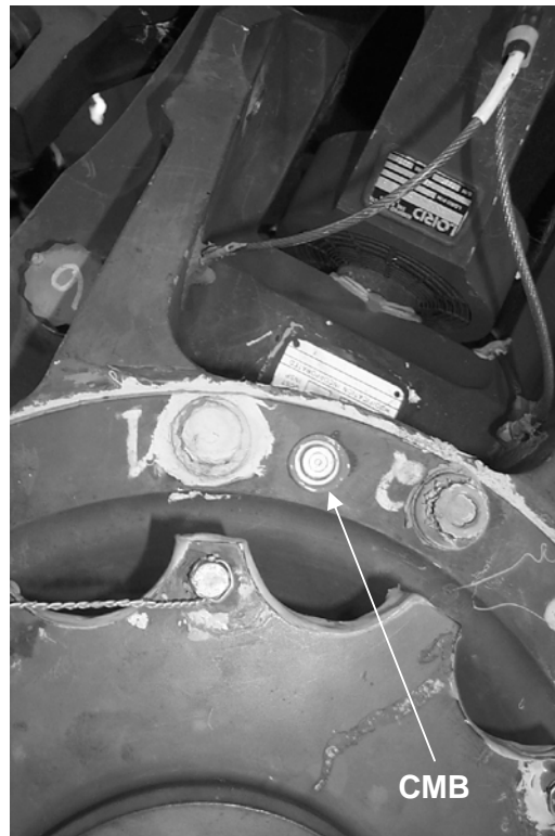
Figure 53. Main Rotor Drive Plate Assembly (AH-64A/D) with CMB Installed
