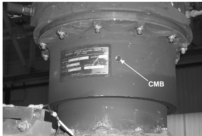
Figure 193. Derotation Unit Assembly (AH-64D) with CMB Installed
